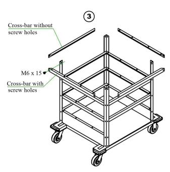
1. Using 2 x M6 bolts attach the cross bars onto the uprights NOTE: Keep these bolts loose
