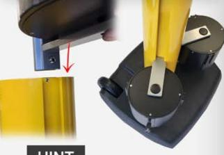
Replace the cap and tighten the three grub screws using the mini screwdriver.
